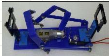
Each Single Motor Robot should be equipped with a 2.1mm socket for the plug of hand generator.
