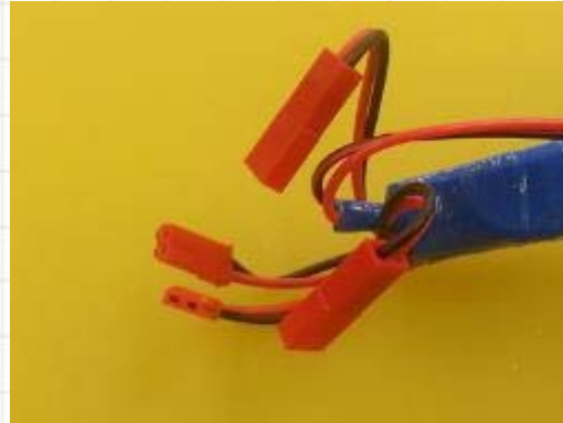
Exchange the plugs to change the polarity and turning direction of handle
