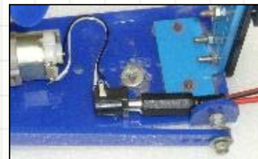
Each Single Motor Robot should be equipped with a 2.1mm socket for the plug of hand generator.
